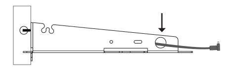
**STEP 7** Plug cable into device.
