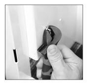
1. Remove nut and remove the ground wire.
