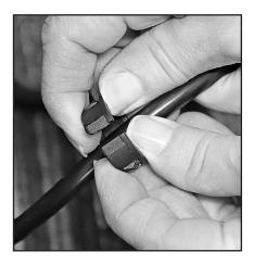
2. Widen the opening in the grommet and feed the power cord through.
