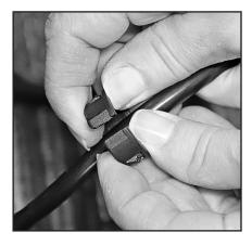
2. Widen the opening in the grommet and remove the power cord.
