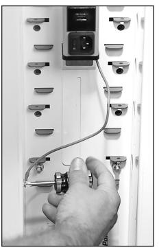
2. Screw the ground wire into the screw on the side of the spine.
