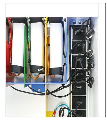
4. Place the prepared power bank into the compartment.
