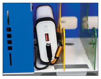
5. Plug black USB-A to USB-C cord into the C port of the power bank to charge.
