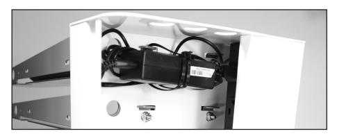
Feed a second zip tie through the hole, then tighten it around the pre-wrapped power brick.
