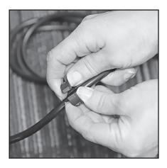
Widen the opening in the grommet and feed the power cord through.
