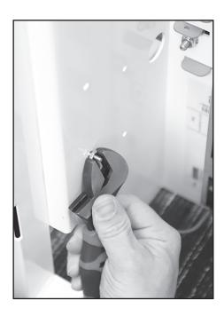
2. Remove old power strip in the back spine of the Tower and set aside.
