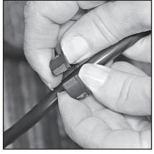
2. Widen the opening in the grommet and remove the power cord.
